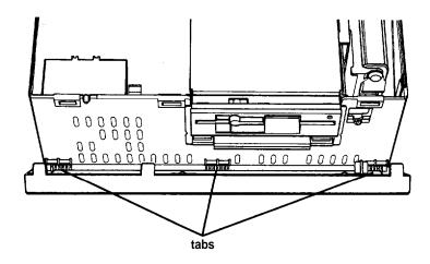
11. Tilt up the front panel until the clips on the top of the panel touch the computer. Then push on the top of the panel until it clicks into place. The diskette drive(s) should be flush with the front panel.
